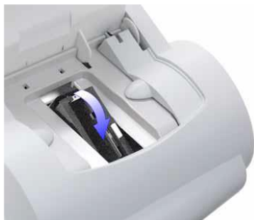
Rotating the Cartridge Compartment
